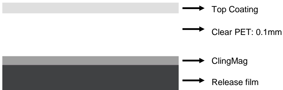
ClingMag Construction Drawing
