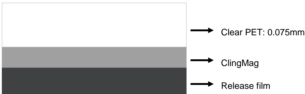
ClingMag Construction Drawing
