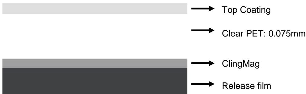
ClingMag Construction Drawing
