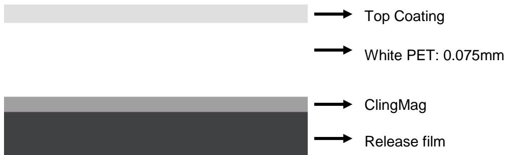
ClingMag Construction Drawing
